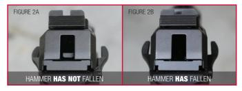
7. If the trigger is blocked and the hammer does not fall, no further action is required, but you should regularly perform this, and all other function checks described in your instruction manual as a part of your normal inspection process.
